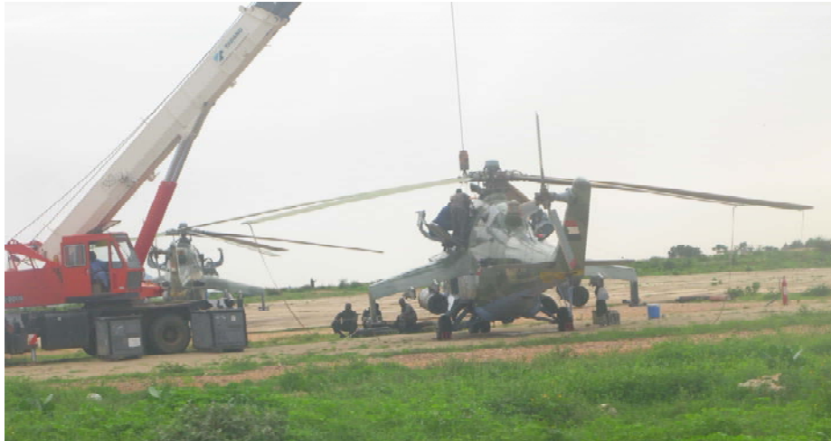
Photo 12 Engine replacement being conducted on an Mi-24 at El Geneina airport, 21 August 2008
